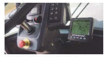
**MODERN, EXACT AND INTELLIGENT** With each compaction pass, the Compaction Meter system indicates when the optimum level has been reached by locating fragile areas, saving time, fuel and money.
